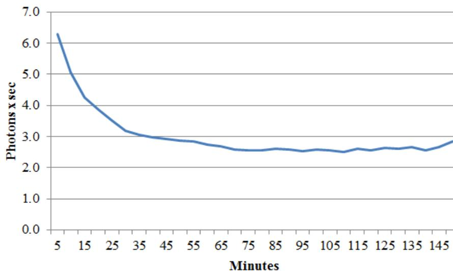
Figure 1: Typical trend of the photons/sec detection rate of the PMT averaged every 5 minutes
