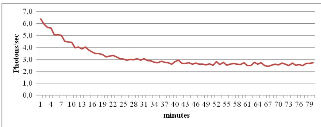
Figure 5: Trend of the photons/sec detection rate during the period of the PMT cooling.
