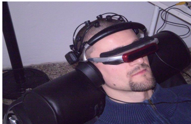
Figure S3: Image of a participant with the complete apparatus: Emotiv™ EEG, digital glasses and headphones.
